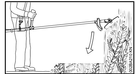
To cut wild growth and scrub, lower the shredder blade down onto the growth to achieve a shredding effect – always keep the cutting attachment below hip level during this process.
