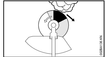
The **risk of kickout is greatest** when the **black area** of the rotating cutting attachment comes into contact with a solid object.
